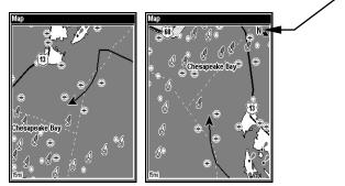
Map orientation is shown in north up (left) and in track up (right).
